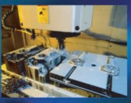
forgings are produced. Every facet of the forging will be machined ensuring the removal of edges that are potential stress raisers. Each rod is rumbled and peened, further reducing potential weakness and giving the ultimate surface hardness and finish.
